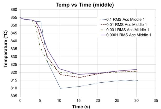
**Figure 7** - Simulation values of a thermocouple welded to the middle of the crucible simulated with different accuracies
