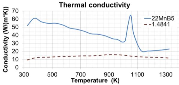
**Figure 2** - The thermal conductivity of 22MnB5 and 1.4841 during the heating cycle
