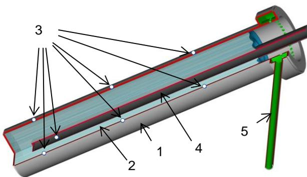
**Figure 9** - Schematic layout of crucible (1) with molten zinc (2), thermocouple positions (3), 22MnB5 sheet metal (4) and propane gas inlet (5)
