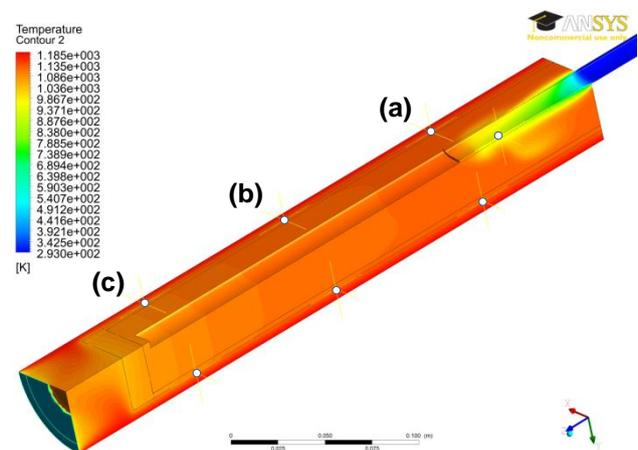
**Figure 11** - Simulated temperature distribution in crucible after 1,5s into the dipping stage
