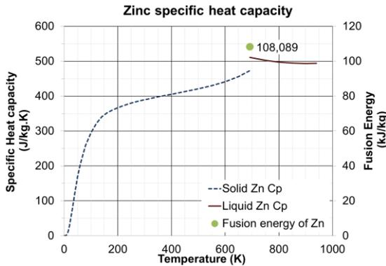
**Figure 3** - Specific heat capacity and fusion energy of zinc [15]
