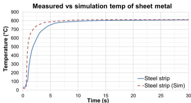
**Figure 13** - Comparison between average measured sheet metal and simulated temperature
