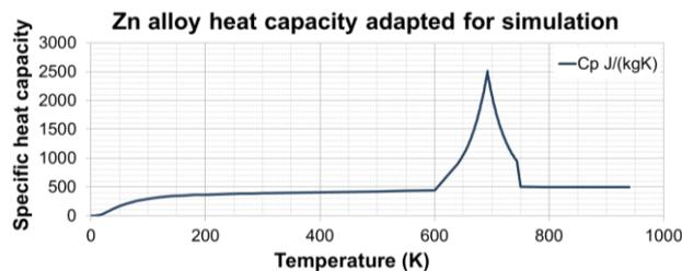
**Figure 5** - Modified specific heat capacity curve of the zinc used in the simulation
