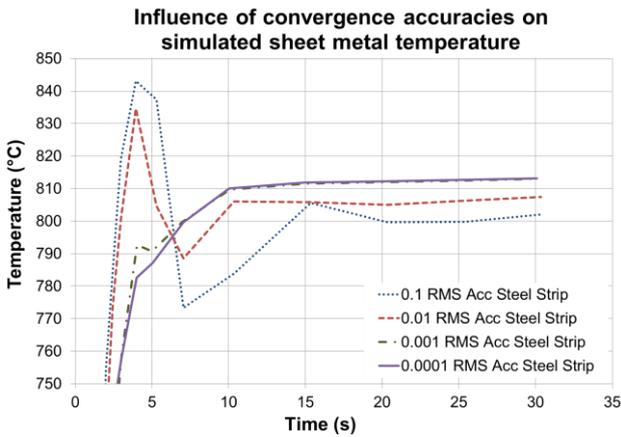
**Figure 8** - Simulated temperature change of thermocouple in the folded 22MnB5 sheet metal
