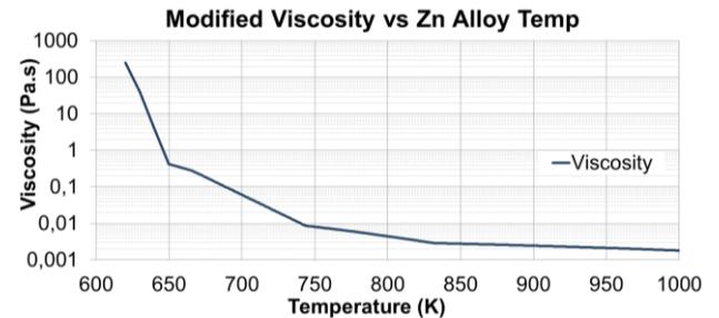
**Figure 6** - Modified viscosity diagram of liquid zinc used in simulation
