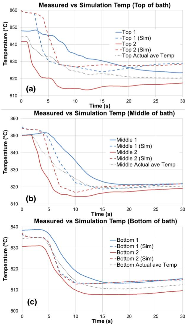
**Figure 12** - Comparison between the measured crucible and simulated temperatures at the 3 different levels
