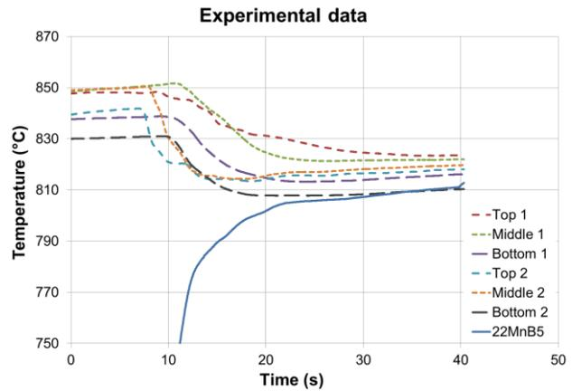
**Figure 10** - Temperature curves from the thermocouples as measured for 22MnB5 1.5 mm thick and 50 mm wide dipped into the zinc alloy
