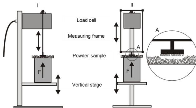
**Figure 3 - Powder tensile test setup**
