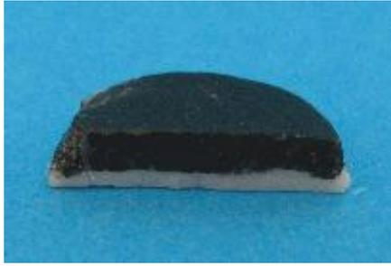
**Figure 8** - Picture of a cut sample with PE-HD powder (on top) and PP powder
