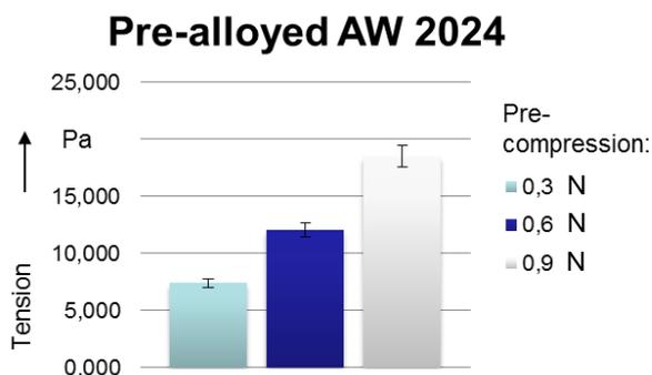
**Figure 5 - Tensions after pre-compressions without nano-particles**
