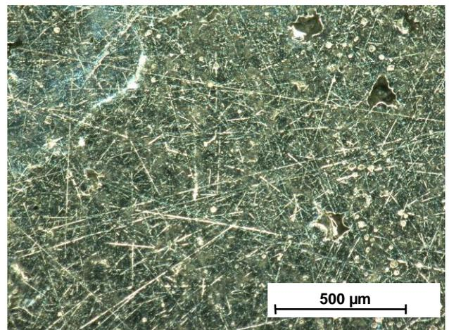
**Figure 6 – Micro-section of Al 6061 after LBM**
