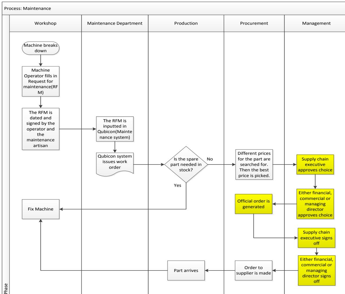
**Figure 6: Maintenance procedure**
