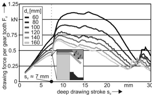
**Figure 6** - Deep drawing forces per gear tooth and shifting of the bending radius.
