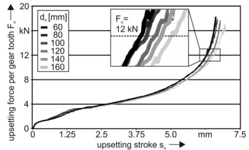
**Figure 9** - Upsetting forces per gear tooth and force value for the mould filling analysis.
