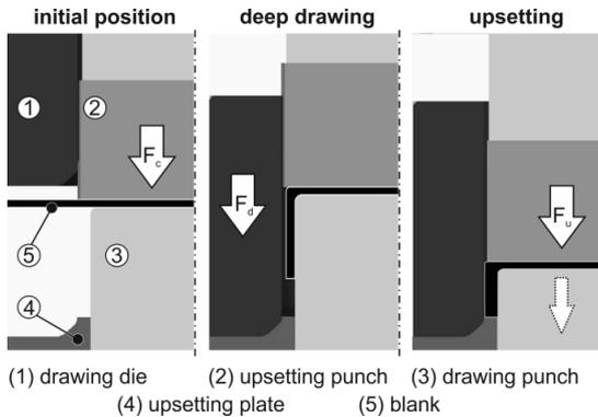
**Figure 2 - Forming sequence and process forces.**
