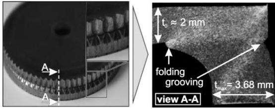
**Figure 4** - Cup with external gearing and sectional view from the experimental set-up.
