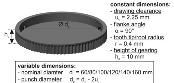
**Figure 5** - Parametric part design.
