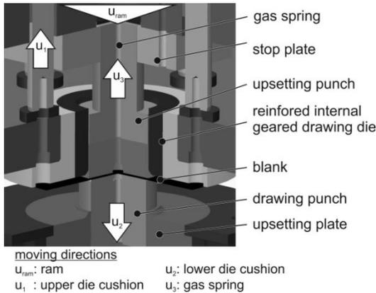
**Figure 1 - Tool set-up and individual tool motions.**
