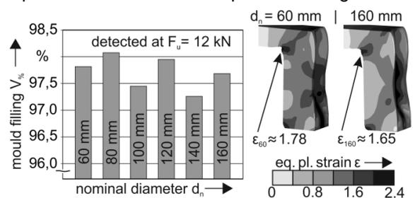
**Figure 10** - Percentage mould filling and deformation characteristics at  $F_u = 12$  kN.
