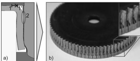
**Figure 11** - Reduction of folding and grooving by the application of tailored blanks.
