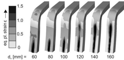
**Figure 7** - Indentation of the gear shape represented by increased local deformation.
