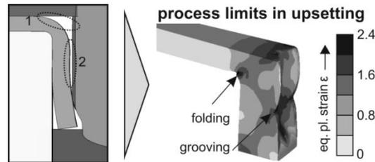
**Figure 3 - Effects of the deep drawing operation on the mould filling in upsetting.**
