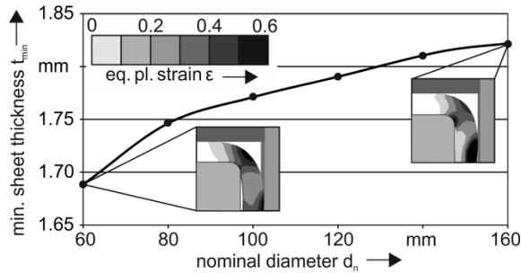
**Figure 8** - Sheet thickness reduction and plastic strains in the fillet after deep drawing.
