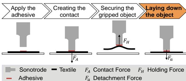
Figure 4 - Sequences of ultrasonic assisted gripping
