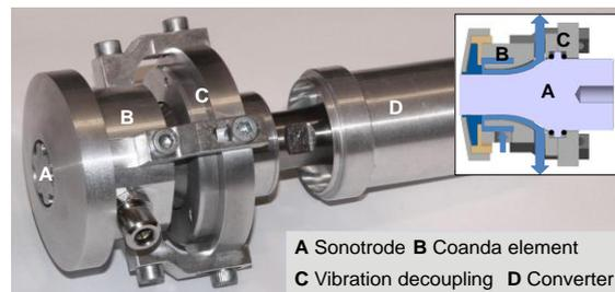
Figure 5 - Prototype and functional principle of the combined gripper.
