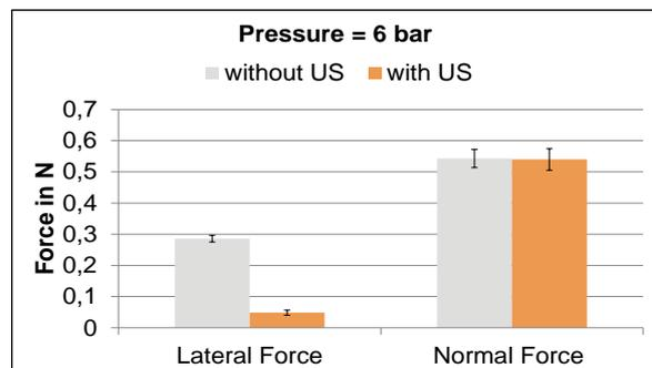
Figure 6 - Measured lateral and normal force depending on ultrasonic vibrations.
