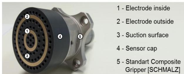
**Figure 7** - Prototype of sensor-based Coanda gripper.
