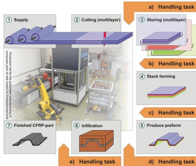
Figure 1 - RTM process and process chain steps.
