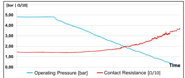
**Figure 8** - Relationship between contact-resistance and the operating pressure.
