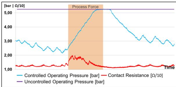
**Figure 10** - Control process to compensate dynamic process forces.
