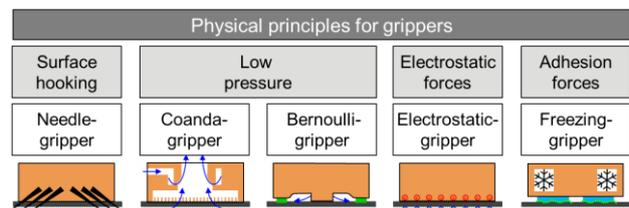
Figure 2 - Typical grippers for textile semi-finished products [8].
