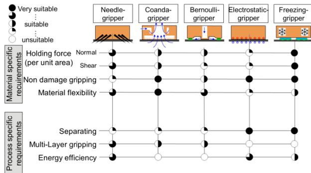
Figure 3 - Evaluation of gripper principles.
