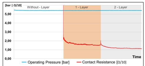
**Figure 9** - Contact-resistance by gripping one, two and no layer of semi-finished textile.
